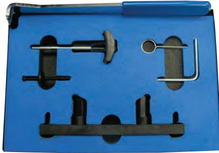
Locking tools also suitable for Scirocco ('09-), Golf VI 2.0R with engine codes CDLA, CDLC, CDLF
